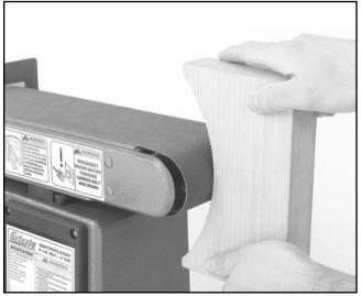
Figure 22. Sanding an inside curve.
